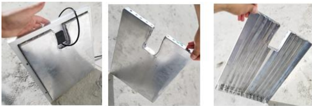
Figure 1. An aluminum container with internal fins attached to the back of the solar panel.
