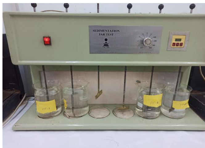
Figure 8. Schematic representation of the jar test setup used for batch adsorption experiments.
