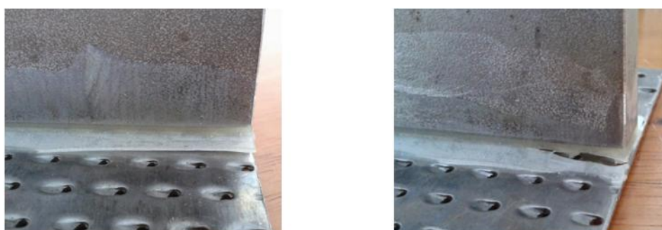
(a) Adhesive failure
