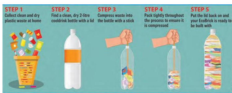
Figure 1. Process flow diagram of the ecobrick production from plastic waste.
