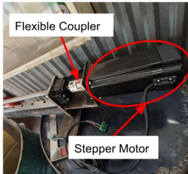
Figure 6. Installation of the stepper motor.
