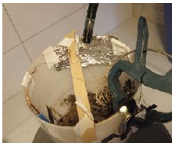
Figure 1. Pot made in plastic, with soil, bog moss, and two electrodes.
