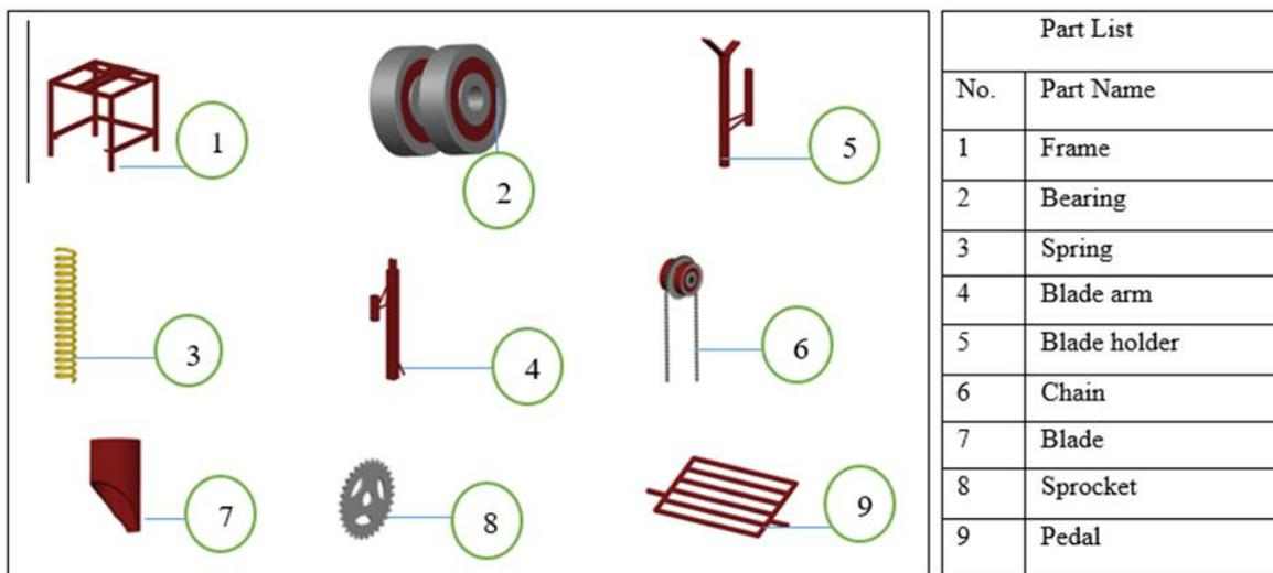
**Figure 8.** Illustration image of the Sugarcane Bud Chipping Machine.
