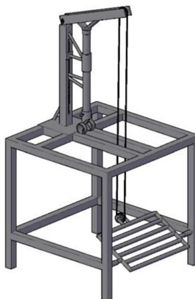
**Figure 11.** Illustration image of Isometric view of the Sugarcane Bud Chipping Machine.
