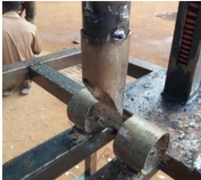
**Figure 7.** Photograph image of the U-shaped Blade.
