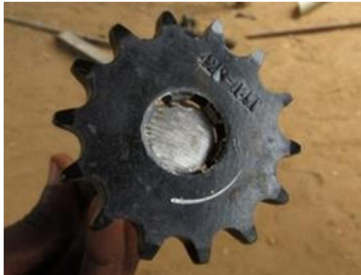
**Figure 5.** Photograph image of the 428-14T Sprocket.
