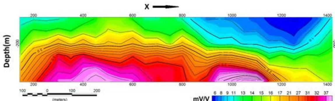
**Figure 14.** Charge ability Pseudo-depth section.
