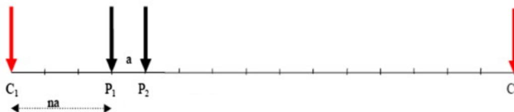
Figure 4. Gradient electrode array.
