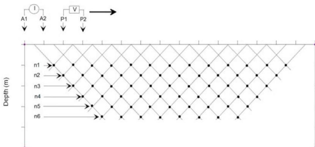
Figure 5. Dipole-dipole electrode array.
