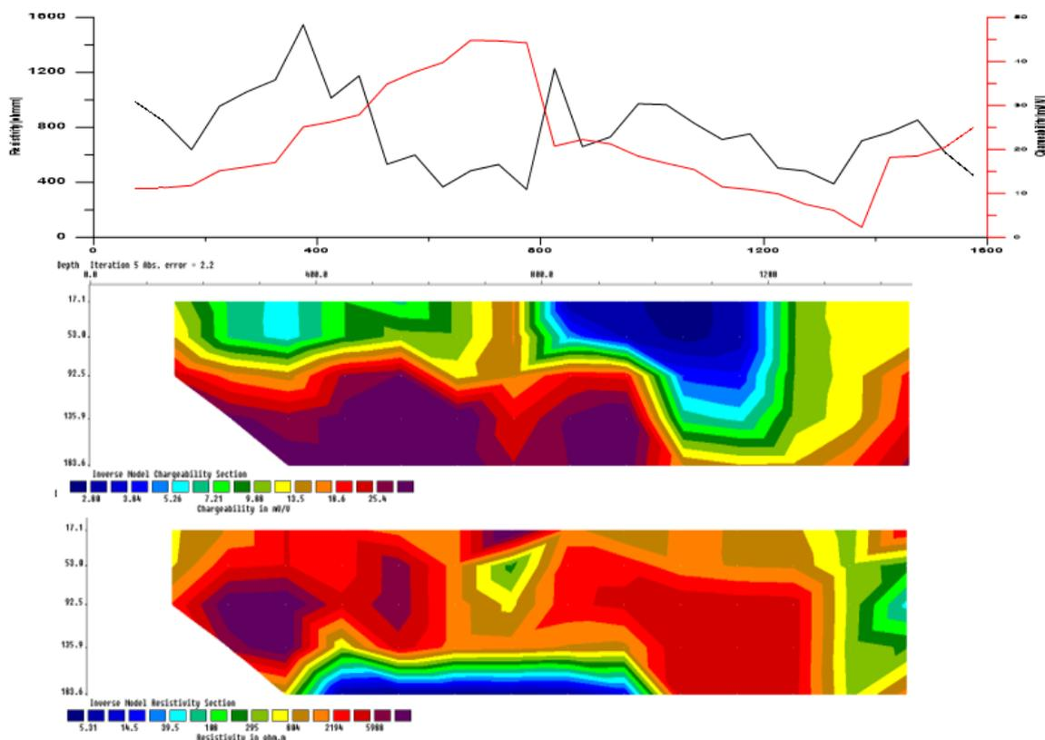
**Figure 15.** Inverted depth sections of resistivity and charge ability.
