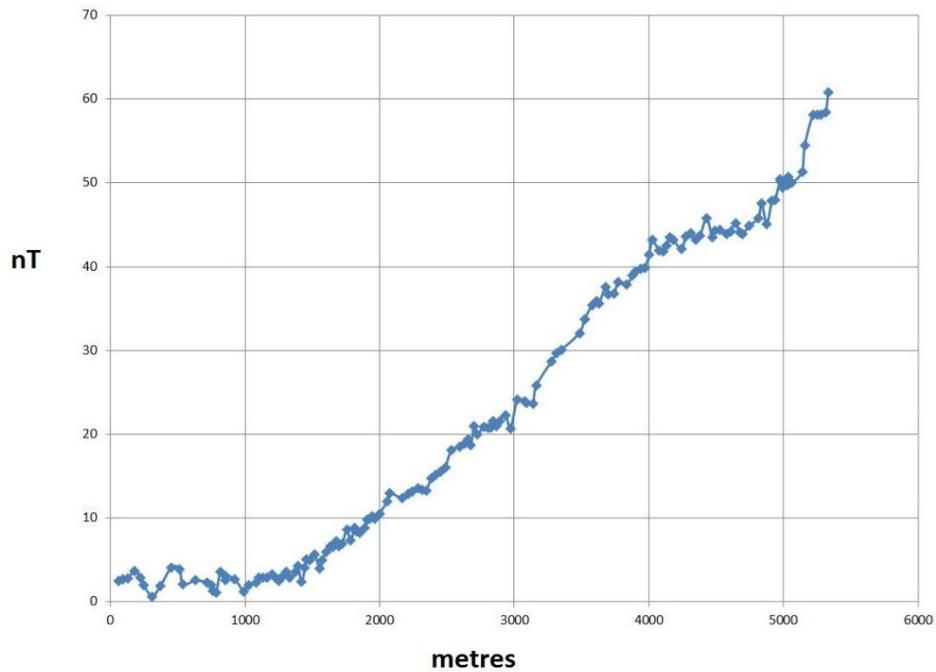
Figure 8. Magnetic anomaly over profile L2.
