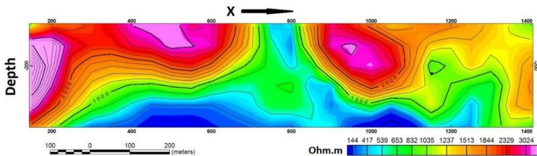
**Figure 13.** Resistivity Pseudo-depth section.
