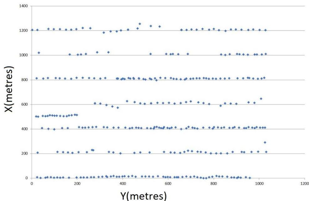
**Figure 3.** Magnetic survey stations layout.
