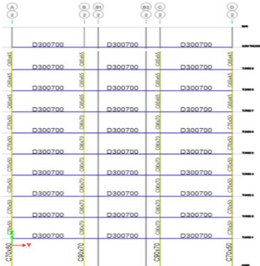
Figure 2. Calculation diagram of Frame Axis 2 in ETABS.
